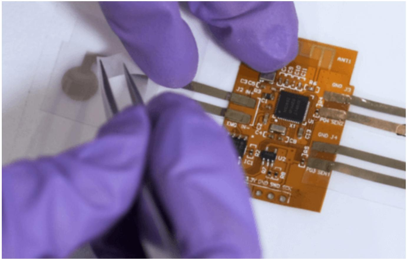
*The BIND interface (biphasic, nano-dispersed interface) makes assembly of stretchable devices simple while offering excellent mechanical and electrical performance.* CREDIT: NTU Singapore
